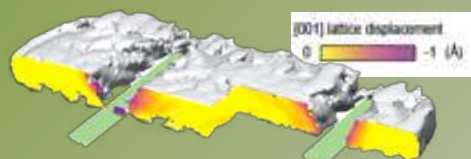
Strain in SiGe device by Bragg ptychography S. O. Hruszkewycz et al. arXiv:1506.01262v1 [cond-mat.mtrl-sci]
