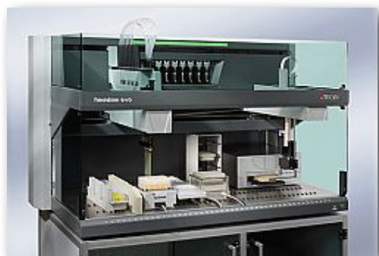
Tecan Freedom Evo 150 reformatting of crystallisation screens
